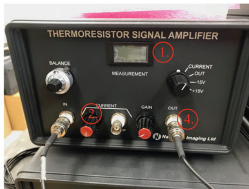
(b) Photo of thermoresistor signal amplifier
