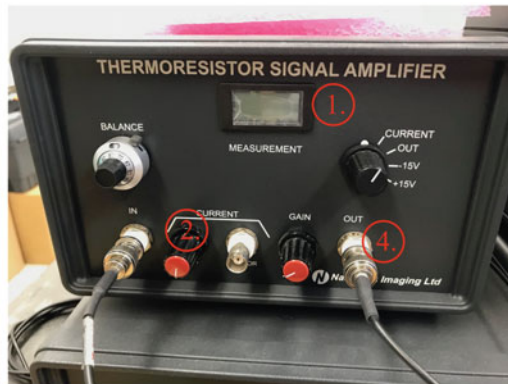
(b) Photo of thermoresistor signal amplifier
