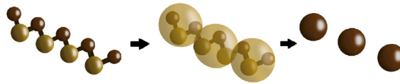
Fig. 1. The idea of CG modeling: the atomistic model (left), the atoms combined to super-atoms (middle), the CG model (right) (adopted from Chen et al. (2011)).
